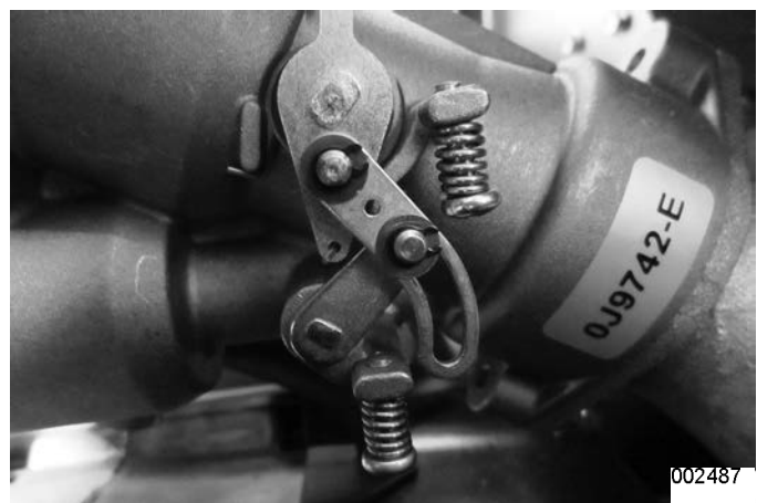
Figure 2-15. Stepper Motor Mid-point = Starting Point, Smaller Venturi Partially Open
