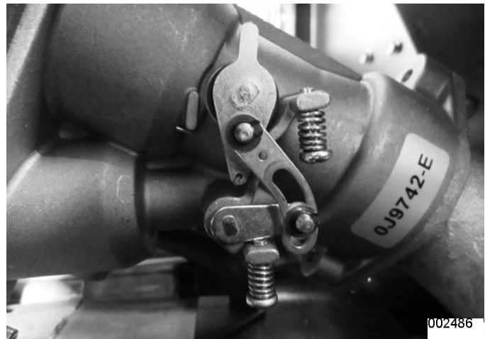
Figure 2-14. Stepper Motor Closed – Closes Both Venturis
